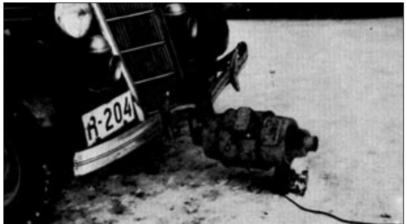
Fig. 2. High voltage generator powered by private car also used for transport of X-ray unit.
